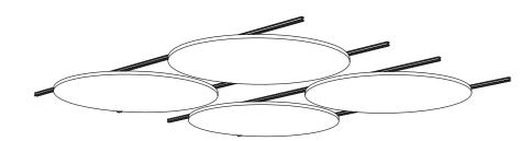
For larger scale installations Horizon can be installed to battens
