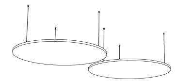
Horizon can be suspended on simple wires
