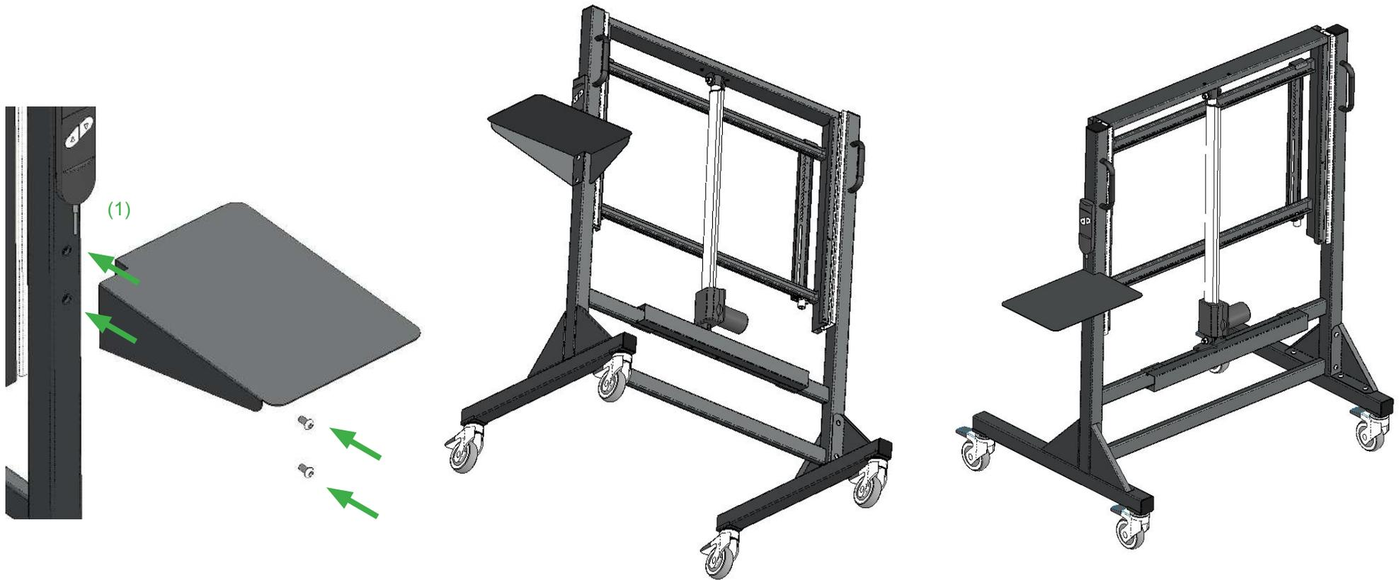
(1) Attach the shelf to the mobile stand with 2 M8 x 16 button head screws. Firmly tighten screws with supplied Allen key.
