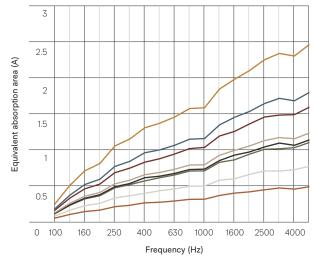
All results are reported in metric sabin - per unit. Equivalent sound absorption area according to ISO 354 measurement of sound absorption in a reverberation room. Average absorption (sabins per unit) calculated at one-third octave bands centred on 250 Hz, 500 Hz, 1000 Hz, and 2000 Hz and rounded to the nearest 0.05.
