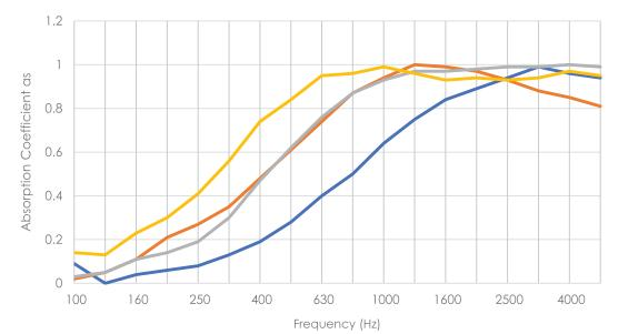
University of Auckland Test Report Number Frequency (Hz) 125 250 500 1000 2000 4000 NRC α<sub>P</sub> 12mm Cube T0712-3 0.05 0.10 0.30 0.65 0.90 0.95 0.45 α<sub>P</sub> 12mm Cube (with 25mm air gap) T0712-6 0.05 0.30 0.60 0.95 0.95 0.85 0.70 α<sub>P</sub> 24mm Cube 0.90 1.00 1.00 0.70 α<sub>P</sub> 24mm Cube rith 25mm air ga 0.80
