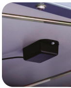
Built-in heat sensor will shut off power if a device overheats.
